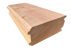
3x6 T&G Douglas Fir **Select Dex** is a commonly used roof decking product in both commercial and industrial applications. With a beautiful appearance and long-span capabilities, Select Dex is an extremely versatile product. Select Dex is 100% Douglas Fir and is profiled with a double T&G and an exposed V-Groove face. It is fully Kiln Dried and available in random lengths from 8' – 20'.
