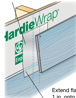
10.9 Flashing behind to add an additional layer of protection from water infiltration
