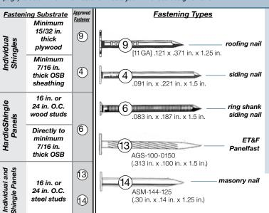
Corrosion-resistant siding nails 1<sup>1</sup>/4-in. long should be used to apply individual HardieShingles® to minimum <sup>7</sup>/16-in.
