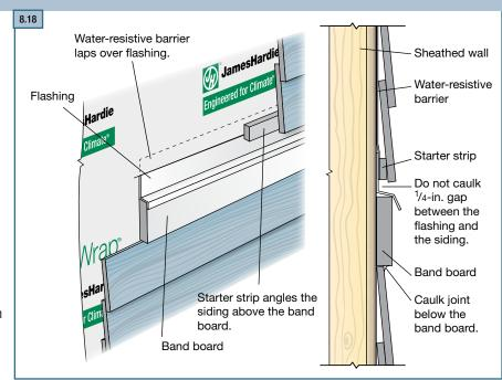
ous drainage plane. If running lap siding or shingle siding above the band board, a starter strip should be installed first to maintain the correct siding angle. Small Periodic gaps should be left in the starter strip to provide an escape route for excess moisture that may drain down behind the siding.
