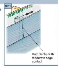
COLORPLUS® TIP: When installing HardiePlank lap siding with ColorPlus Technology, position the plank in the immediate area where the plank is to be fastened. Do not place the plank on the course below and slide into position. Doing so may scuff or scratch the ColorPlus finish on the installed piece.
