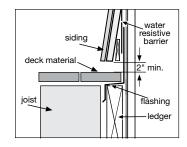
At the juncture of the roof and vertical surfaces, flashing and counterflashing shall be installed per the roofing manufacturer's instructions. Provide a minimum 2" clearance between the roofing and the bottom edge of the siding and trim.
