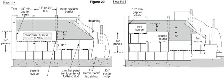
position nails on nail line and secure into framing. Only when application is to minimum 7/16" thick APA rated sheathing, position nails on nail line spaced a maximum of 13 3/4" o.c. Allow 3/8" from panel edges.
