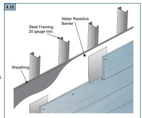
When using a screw to attach James Hardie products to steel, a screw with a self tapping point should be used. A self tapping screw functions by having a cutting edge which drills away the material, making a tiny hole for the screw to go into. Some self tapping screws may be wing tipped which are intended to bore out the fiber cement (creating a pilot hole), and will break off as the screw goes into the steel. Either type of screw is acceptable for use.
