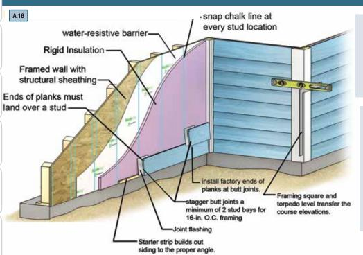
Note: When attaching lap siding products over foam the length of the chosen fastener must be extended by the thickness of the foam to achieve the same required holding power.
