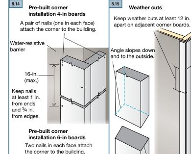
NOTE: All weather cut joints should be touched up prior to installation.
