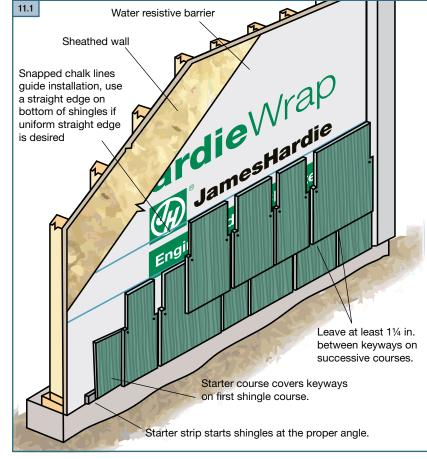
TIP: For the best appearance, apply shingle widths in a random manner to avoid creating a repeat pattern. Pre-planning of each course is recommended to aid appearance and to avoid stacked seams.
