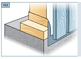
TIP: Install flashing over the footing/foundation and extend the panel over the flashing just below the sill plate. Do not extend siding beyond the required grade clearances. TIP: For Sierra 8
