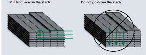
TIP: When taking planks from the pallet installation, avoid repeating the texture pattern by working across the pallet. Two to four planks can be removed from a stack at one time. But then material should be taken from adjacent stacks, again working across the pallet. Texture repeat is typically a concern on large walls with few breaks, such as windows or doors.
