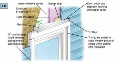
Note: It is recommended to layout the rigid foam insulation such that vertical joints do not occur at the corners of window and door openings or overs if possible.
