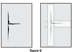
slide HardieWrap weather barrier under slit
