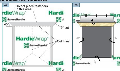
HardieWrap® Flex Flashing should be applied over the water-resistive barrier after it has been cut and set into and around the window rough opening. Refer to installation of HardieWrap® Pro-Flashing and Flex Flashing for flashing guidelines.
