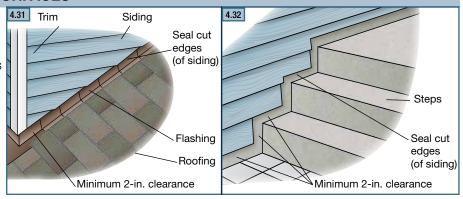
IBC Code Reference: "1503.2.1 Locations. Flashing shall be installed at wall and roof intersections, at gutters, wherever there is a change in roof slope or direction and around roof openings..."
