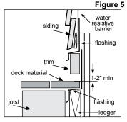
At the juncture of the roof and vertical surfaces, flashing and counterflashing shall be installed per the roofing manufacturer's instructions. Provide a 1-2" clearance between the roofing and the bottom edge of the trim.
