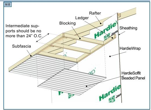
TIP: Stainless steel fasteners are recommended when installing James Hardie products near the ocean, large bodies of water, or in very humid climates.
