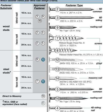
\*When blind fastening 9.5 in. or wider product onto steel studs, use screws.
