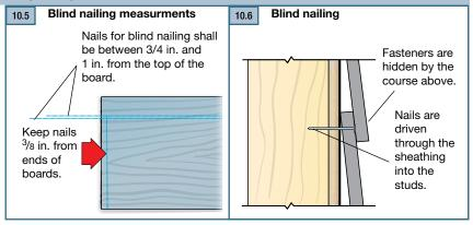
plank. Additionally fasteners should be placed no closer than 3/8 in. from the ends of the plank.
