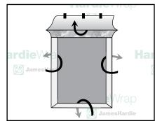
Step 3: Fold the remaining three flaps in through the opening, fastening them inside with staples (fig. 5).
